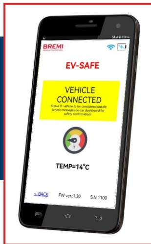
Thanks to the Point-to-Point Wi-Fi connection, the user can directly access the local mini-site to view information on the **vehicle's security status** without having to install a specific App!
